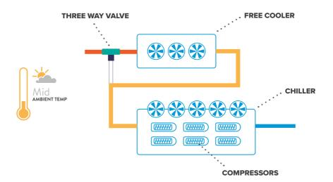
As the ambient air temperature continues to fall, the amount of process heat taken out of the process fluid by the air increases, progressively reducing the load on the chiller. At 5°C below the process supply fluid temperature, all the process heat is removed by the ambient air in the free cooler – providing full free cooling.
