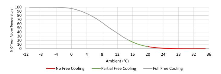
However, even existing free cooling systems can be fine-tuned to make even greater savings. For example, if an operating system is above 10°C, raising the temperature by an extra 1°C won't affect the operation, but will enable a more efficient design as the operating temperature is closer to the ambient air temperature, which makes free cooling a more viable option for providing the bulk of the cooling required.
