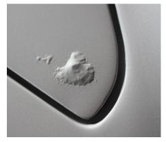
The evidence of SRB attack shows as a pit on the surface of typically mild and stainless steel. SRB in general grow by using a carbon source as energy and then by reducing sulphate common in water to hydrogen sulphide (H2S). It is to be noted that additional nutrients in water also act
