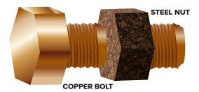
Electrons flow continuously from the most reactive metal (the anode) to the less reactive metal (the cathode) thus fuelling the corrosive process. This potential difference causes electrons to migrate across two dissimilar metals. Below is a simple diagram of this electrochemical process:
