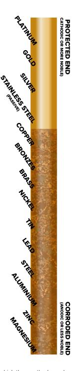
The pathway in which these cathodes and anodes connect is via the type of electrolyte medium, which will accelerate this process, e.g., the higher the conductivity of the water the quicker  $\boldsymbol{\theta}$  more reactive the process.
