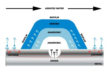
The second Direct MIC is with a bacterium synonymous with this phenomenon: Sulphite Reducing Bacteria (SRB). Once an SRB is present and the correct environment is stable enough for its growth, we can see a rapid and damaging effect. SRB relies on the absence of oxygen; we have seen this where biofilm is present previously. This is because such bacteria are known as anaerobic, where they grow in the absence of oxygen.
