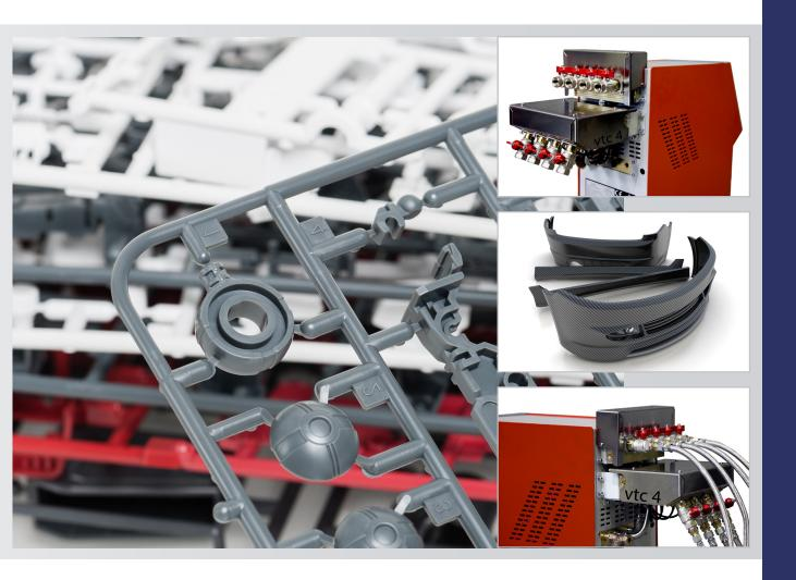
Add-on Manifold with flow and temperature monitoring
