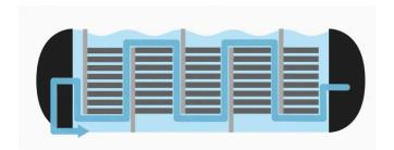
Some further advantages of a flooded evaporator include better flow distribution because the inlet is 100% liquid, better utilisation of the plate area and higher coefficient of performance (COP).
