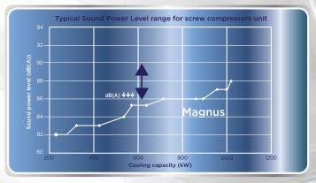
The main functions of the EC fan include a noise reduction level of 4-5dB(A) as well as an absorbed power reduction by 15%. Furthermore the EC fan offers low inrush currents and can also modulate the rotational speed providing reduced noise emissions and maximum energy consumption.
